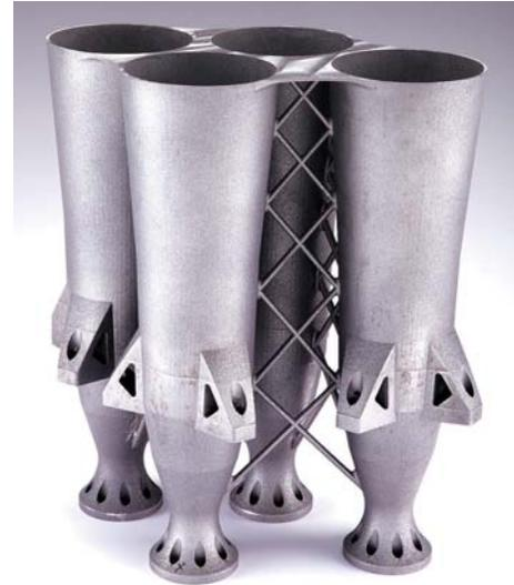
‘Feed Cluster Antenna’ printed in aluminium by Wipro 3D for ISRO. The antenna was part of the GSAT-19 satellite’s communication system
